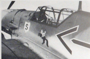
Detail of non-standard octane triangle
