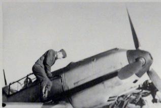
LEFT: By the beginning of 1940, Luftwaffe fighter units had begun to adopt a modified camouflage scheme with a splinter pattern of dark-green (RLM 71) and RLM Grey (RLM 02) on the upper surfaces with light blue (RLM 65) on the fuselage sides and underneath. This eventually proved too conspicuous and began to be overpainted with grey or green or combinations of both once the spring weather started to break. This BF 109 E-1 of II (J)/Tr Gr 186 is being readied for action at Nordholz airfield and still carries the large crosses under the wings introduced in October 1939 (see Section 3 page 276 for more details).
