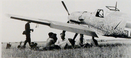
ABOVE: The ground crew of this Bf 109 E-1 coded Red 7 (outlined in white) of 8/JG 2 take a break from servicing their aircraft. The paintbrush stipple finish is very evident and, on this machine, the Balkenkreuz has not been modified. Note that the stipple has been taken down to include the wing root itself! The aircraft also carried the JG 2 Geschwader emblem as well as the 8. Staffel badge on the nose which was part of the family crest of the Staffelführer, Obit Alexander von Winterfeldt.
