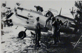
LEFT: Mechanics of 2./JG 3 based in the Bonn area prepare this Bf 109 E-3, coded 'Black 4' for a mission in the west at the beginning of 1940. An interesting feature on this aircraft is the number '4' painted around the '87 octane triangle' (marking the fuel filler position). This aircraft was painted in similar colours to the Bf 109 Ia described opposite and again no unit identity emblems had been applied at this time. The aircraft is camouflaged in the splinter pattern on the upper surfaces of dark-green (RLM 71) and RLM Grey (RLM 02) with light blue (RLM 65) on the fuselage sides and underneath.
