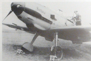
RIGHT: This pilot, an Obergefreiter, with his Bf 109 E-5 of 3./JG 3, is inspecting his flying helmet in preparation for a flight. The aircraft was camouflaged in standard splinter pattern of that time: with dark green (RLM 71) and RLM grey (RLM 02) on the upper surfaces and light blue (RLM 65) on the fuselage sides and underneath. The 3. Staffel badge is clearly visible below the cockpit and the aircraft also has a personalised inscription 'Fortuna' (fortune) painted on the nose. The spinner and propeller are in the standard colour of black-green (RLM 70).
