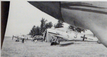
LEFT: BF 109 E-3s including 'Brown 5' and '4' (outlined in black) of 6./JG 26 stand ready for action on a makeshift airfield in France during late June 1940. The aircraft carry the JG 26 'Schlageter' emblem as well as the 6./JG 26 'Steinbock' badge and look to have received only very slight staining around the engine exhausts. It would appear that the spinners may also be painted brown (RLM 26). The groundcrew have established themselves under canvas knowing that the fighting is almost over and it appears that some transport has been acquired ready for some anticipated leave.
