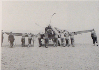
ABOVE: This Bf 109 E-1 of 6./JG 26 made a belly landing, in early spring 1940, with the engine still running as indicated by the shape of the propeller. The mechanics have managed to raise the aircraft using an air bag, which, when put underneath the machine lifted it off the ground and allowed the lowering of the undercarriage. The deflated bag can be seen stowed on top of the wing. The machine is being pushed off the airfield towards the repair workshop.
