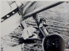
RIGHT: Close-up of the damaged undercarriage of 'White 5' giving considerable detail of the wheels and undercarriage legs
