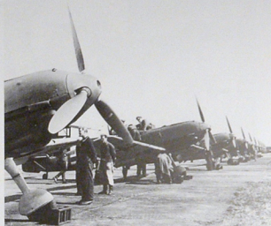
ABOVE: A line-up comprising a mixture of brand new BF 109 E-1s and E-3s stand in a perfect row outside the assembly plant in Augsburg awaiting delivery. The Luftwaffe personnel are looking over the aircraft prior to acceptance to their front line unit. The aircraft will have their basic primer colour on the upper surfaces and fuselage sides. No unit markings have as yet been applied.
