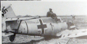
RIGHT: The starboard view of Oblt. Robitzsch's Bf 109 E-1 showing the camouflage demarcation on this side of the fuselage. Note the aircraft still has the Hakenkreuz carried over the fin and rudder. The aircraft was camouflaged in a standard splinter pattern of dark green (RLM 71) and RLM grey (RLM 02) on the upperparts with light blue (RLM 65) on the fuselage sides and underneath. The aircraft also carried a black band outlined in white, the same width as the code number, running right around the fuselage.
