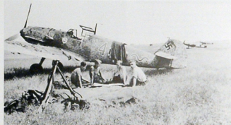
ABOVE: With the fuselage Balkenkreuz covered as camouflage from the air, the ground crew, with weapons in hand, take a break in front of Uffz. Georg Hippel's Bf 109 E-1 coded Red 7 outlined in white with the III Gruppe way line in red after the fuselage cross. The brush stipple finish applied to the fuselage is very evident as is the JG 2 emblem and the 8. Staffel badge.
