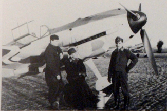
LEFT: What appears to be a brand new BF 109 E-3 just delivered to II (J)/Tr Gr 186 around early March 1940, though the aircraft still has the large 1939 national markings on the underside of the wings. The aircraft appears to carry the number 'Red 5' outlined in white and also has the new 'square' canopy top which was a modification providing simpler manufacture than the original rounded top. The spinner and propeller were painted black-green (RLM 70) and the rest of the aircraft carried a splinter pattern of dark-green (RLM 71) and RLM Grey (RLM 02) on the upper surfaces with light blue (RLM 65) on the fuselage sides and underneath.
