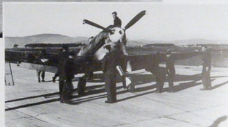
LEFT: This BF 109 E-3 probably belonging to 5/JG 77, stands on a timber boarded runway. As timber was a readily available construction material in Scandinavia, it was used to make handboardings and runways for aircraft. This machine appears to have received a new rudder and the mottling on the fuselage has been applied much less heavily except for the nose.
