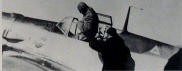
ABOVE: The new Kommandeur of II./JG 77, Major Harry von Bülow-Bothkamp, clambers into the cockpit of his Bf 109 E-3 at Jever on the German flight at the beginning of 1940. The aircraft is camouflaged in splinter pattern on the upper surfaces comprising dark-green (RLM 71) and RLM Grey (RLM 02) on the upper surfaces with light blue (RLM 65) on the fuselage sides and underneath. By this time the old seagull emblem of II./JG 77 had been replaced by an eagle's head flying over the sea.
