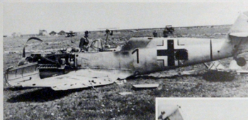
RIGHT: The starboard view of Oblt. Robitzsch's Bf 109 E-1 showing the camouflage demarcation on this side of the fuselage. Note the aircraft still has the Hakenkreuz carried over the fin and rudder. The aircraft was camouflaged in a standard splinter pattern of dark green (RLM 71) and RLM grey (RLM 02) on the upperparts with light blue (RLM 65) on the fuselage sides and underneath. The aircraft also carried a black band outlined in white, the same width as the code number, running right around the fuselage.
